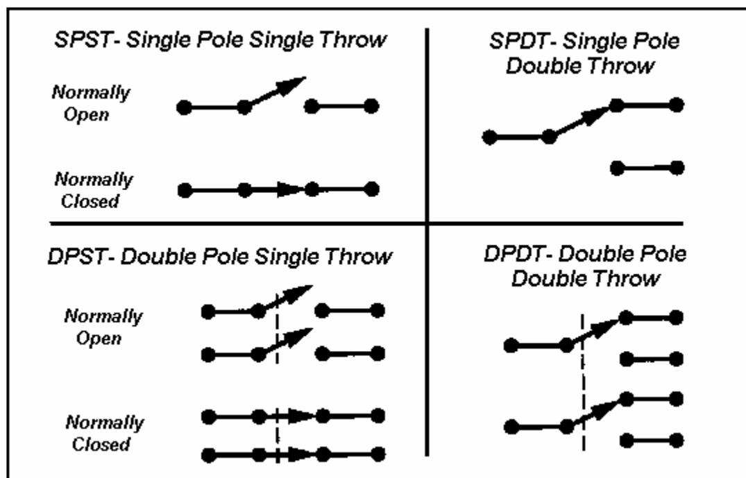
Some audio companies use toggle or rotary switches to select the audio source by sending the audio signal through the switch. While it is a cheap way to route audio signals, it also tends to add a significant amount of noise into the system. We highly recommend avoiding this application.
